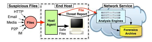
Figure 3: Architectural approach for in-cloud file analysis service.
