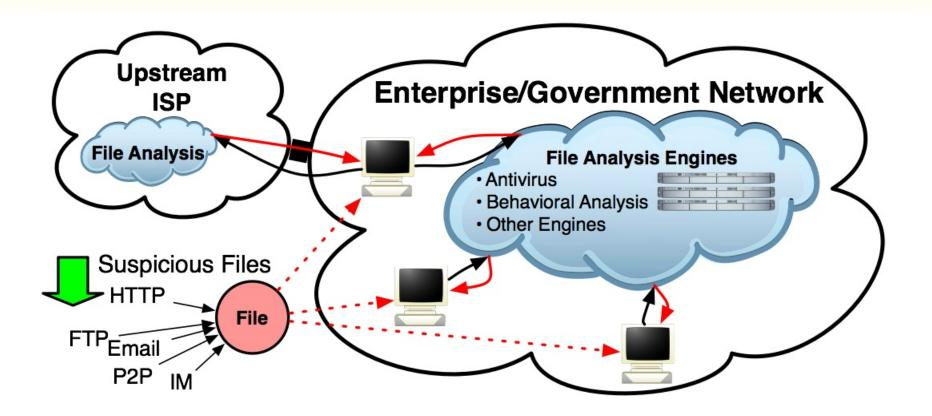
Network service can be deployed inside an organization or by an upstream ISP
